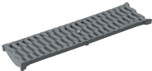
Slotted steel grating, OvalGrip Design, plastic, gray Load class: B125 , Lenght: 50 cm, SW 8 mm
