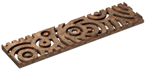
Design grating, CELTIC, cast iron, uncoated Load class: C250 , Lenght: 50 cm, SW 10 mm
