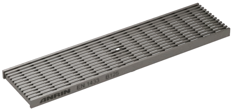
Longitudinal profile grating, stainless steel Load classes: B125, D400 , Lenght: 50 cm, 100 cm, SW 5 mm
