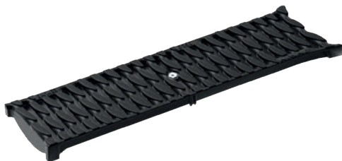
Slotted steel grating, OvalGrip Design, plastic, black Load class: C250 , Lenght: 50 cm, SW 8 mm
