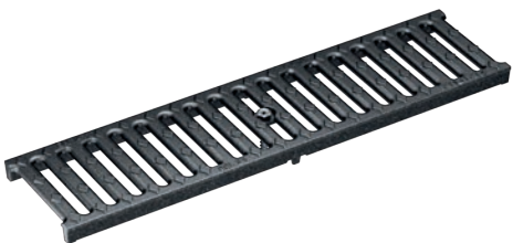
Slotted steel grating SW 10, cast iron, cataphoretic dip coating Load class: C250 , Lenght: 50 cm, SW 10 mm
