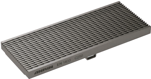
Longitudinal profile grating, stainless steel Load class: C250 Lenght: 50 cm, 100 cm, SW 5 mm
