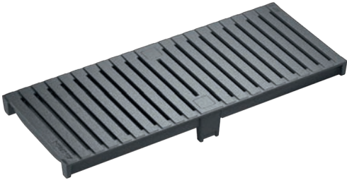
Slotted steel grating, HEELGUARD, cast iron GJS, coated in black Load class: D400* Lenght: 50 cm, SW 6 mm
