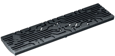
Cast iron grating, WIRE Design, cast iron, cataphoretic dip coating Load class: D400* , Lenght: 50 cm, SW 5 mm
