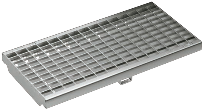
Mesh grating, galvanised, stainless steel Load classes: C250 , D400* , Lenght: 50 cm, 100 cm, MW 30 x 20 mm / 20 x 20 mm
