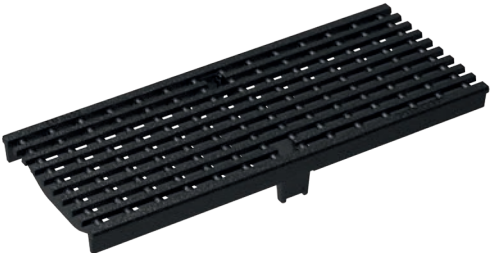
Longitudinal-bar grating, cast iron GJS, cataphoretic dip coating Load classes: D400*, E600* Lenght: 50 cm, MW 25 x 11 mm
