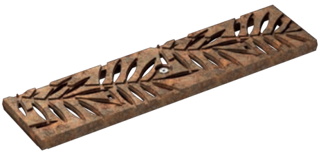
Design grating, LEAF, cast iron, uncoated Load class: C250 , Lenght: 50 cm, SW 5 - 9 mm
