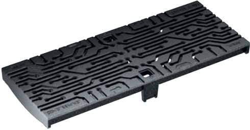
cast iron grating, WIRE Design, cast iron GJS, cataphoretic dip coating Load class: D400* Lenght: 50 cm, SW 5 mm
