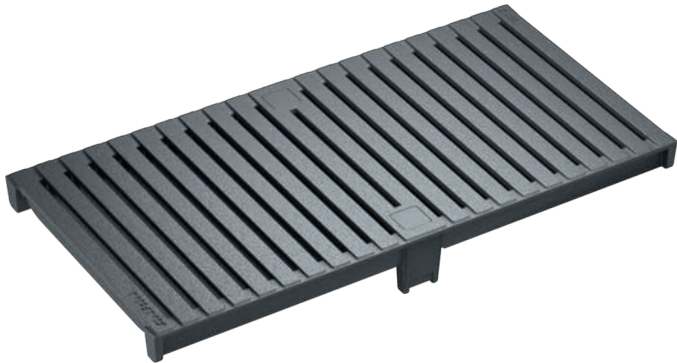
Slotted steel grating, HEELGUARD, cast iron GJS, cataphoretic dip coating, coated in black Load classes: D400* , Lenght: 50 cm, SW 6 mm
