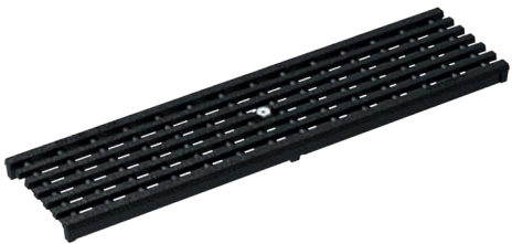
Longitudinal-bar grating, cast iron, cataphoretic dip coating Load class: D400* , Lenght: 50 cm, MW 25 x 10 mm
