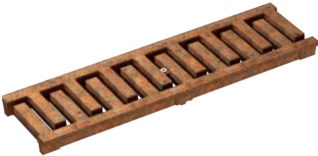
Slotted steel grating, MASSIV 32, cast iron, uncoated Load class: E600* , Lenght: 50 cm, SW 11 mm Only suitable for KE-100.
