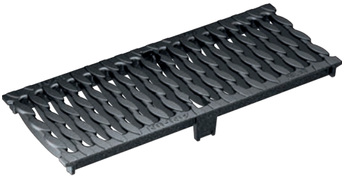
cast iron-Slotted steel grating with OvalGrip Design, cast iron GJS, cataphoretic dip coating Load classes: D400*, E600* Lenght: 50 cm, SW 12 mm
