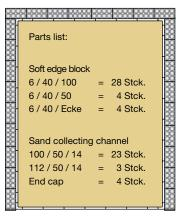
Installation plan for long jump pit edging based on a pit with dimensions of 9.00 x 7.00 m.
