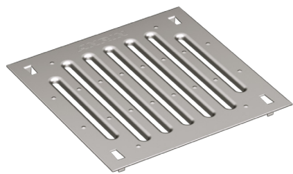
Slotted grating Material: galvanised steel Length: 25 cm Load class: A15
